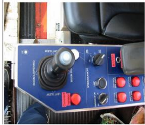
Stb crane, new panel with joy stick 324 0448-801 (Slewing/luffing)
