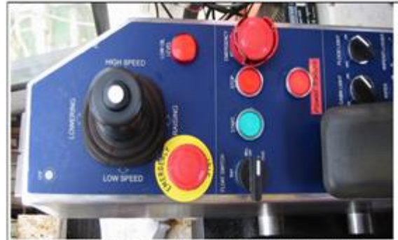
Stb crane, new panel with joy stick 324 0447-801 (hoisting)
